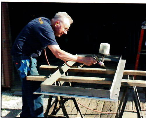
MRM member John Downing is applying a coat of primer paint on the cab door frame he had fabricated to fit on the engineer's door.
