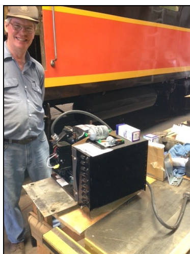
Member Bruce Backus is preparing to install one of four new refrigeration compressors .
