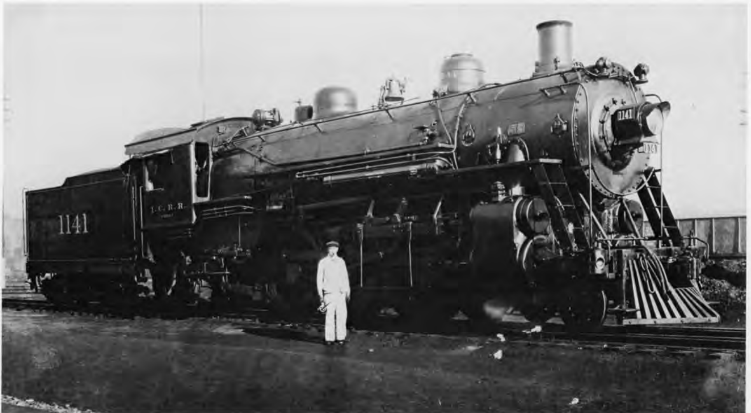
#1141 before improvements, with the original small tender, spoked wheels, etc....
