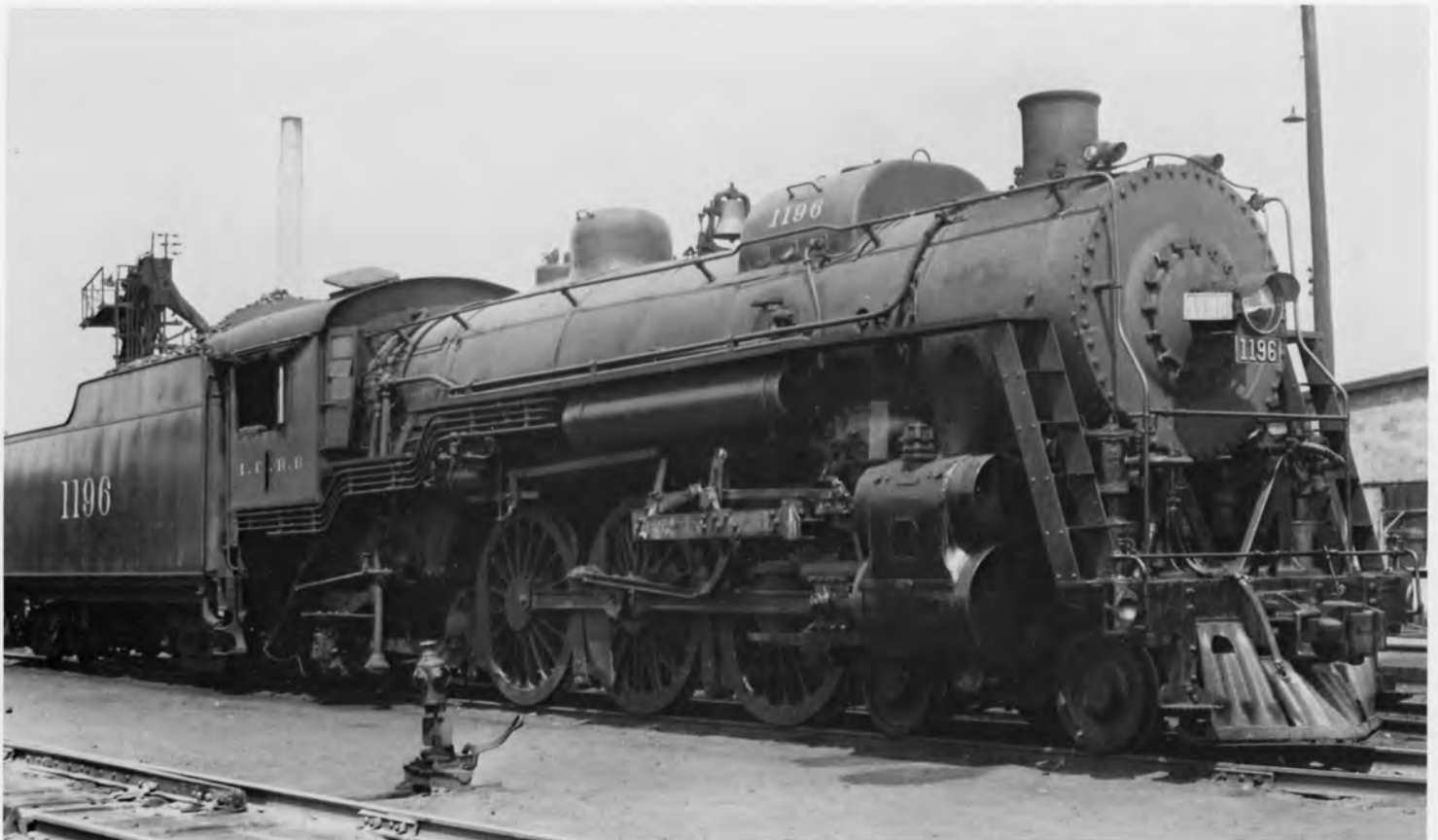
#1196 was one of the engines that got the full modernization treatment at Paducah; corrugated pilot, sand dome, front mounted air pumps, cast pilot wheels, and an enlarged tender.
