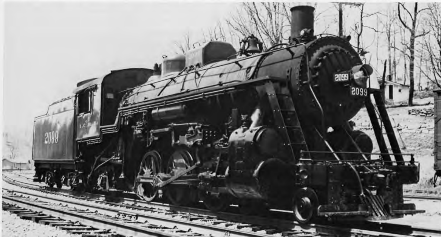
#2099 - The Rogers 2-6-2 that was rebuilt into a Low Wheeled Pacific by the I.C., seen here at Horse Branch KY in 1957. Photo by Jerry Carson
