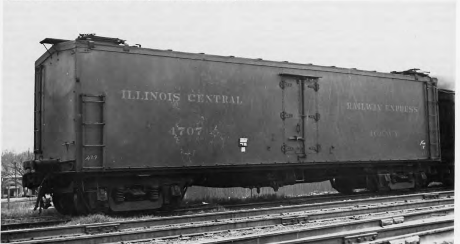
Illinois Central Steel Frame refrigerator car #4707 at Jackson MS 3-20-45 Note passenger car lines and diaphragm buffer. Jerry Carson photo.
