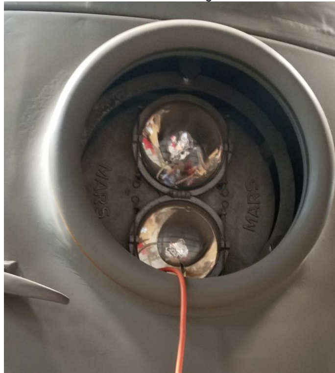
Side body panels are being installed on the engineer side of the unit and a brand new Mars light has been installed.
