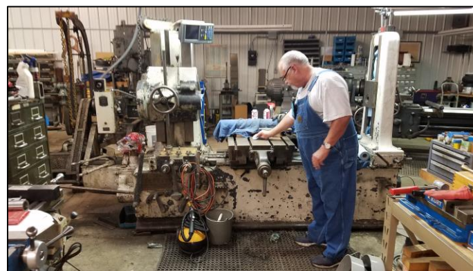
Member Scott Wetter is in the process of improving the mechanical functions of this 1913 Lucas Model 31 Horizontal Boring Mill. With tools of this type, major work can be accomplished in the restoration of equipment.
